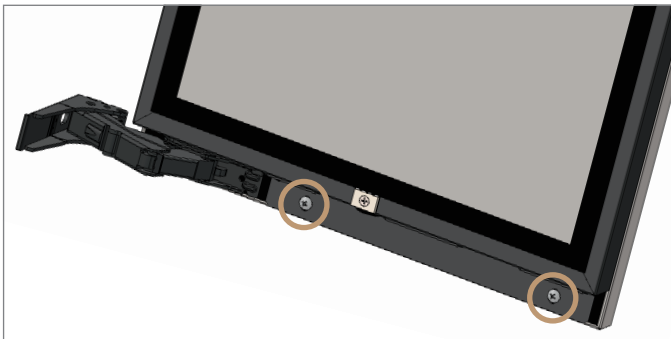
FIG. 2. Bottom door bracket screw locations.
