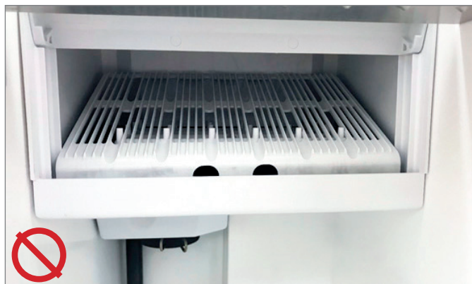
INCORRECT. Ice guide positioned too far inside the water trough.
