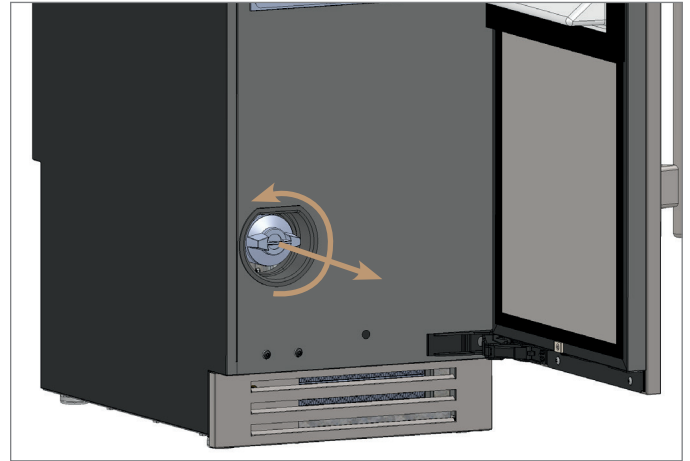
FIG. 1. Rotate the existing water filter counterclockwise.
