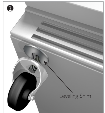
For leveling, insert the shim between the castor and frame rail.
